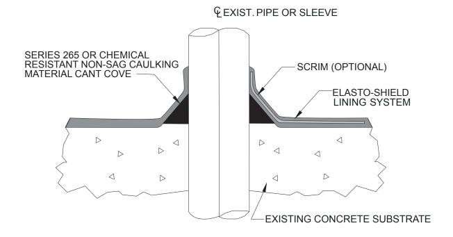
NOTE: ESTABLISH DEEPER SURFACE PROFILE 1" AROUND O.D. OF PIPE PENETRATION TO LOCK LINING SYSTEM INTO SUBSTRATE.
