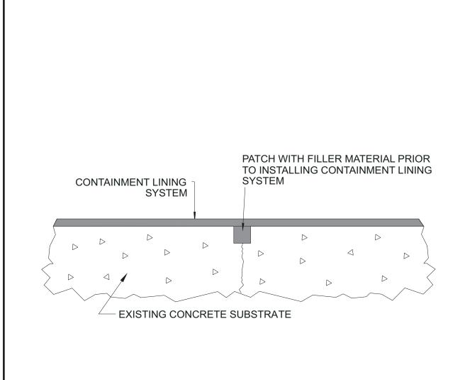
NOTE: USE SERIES 215 OR SERIES 201, 237SC, 239SC 100% SOLIDS EPOXY MIXED WITH FUMED SILICA, SILICA FLOUR OR FINE AGGREGATE FOR FILLER MATERIAL. FILL CONTROL JOINT PRIOR TO INSTALLING CONTAINMENT LINING SYSTEM.
